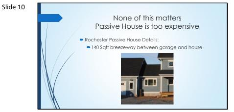
The breezeway helps add an air lock entry, and keep the garage attached to the house. Since Passive House doors are so heavy, they don't make them spring loaded – you'd lose a finger or 2. we needed the spring loaded fire door to have the garage attached to the house.
