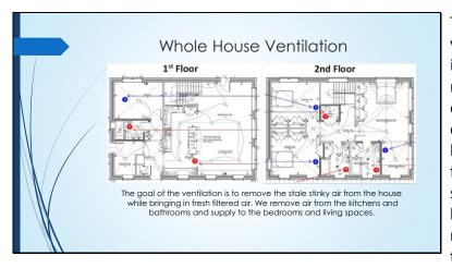
The goal of passive house ventilation is to ensure optimal indoor air quality while maintaining comfort and energy efficiency. Typically we want to exchange all of the air in the house every 3 hours. We bring in fresh filtered air and exhaust the stale stinky air. This is done with heat recovery to ensure we maintain the indoor air temperature.
