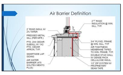
Window installation detail, connecting the air barrier to the window frame is very important
