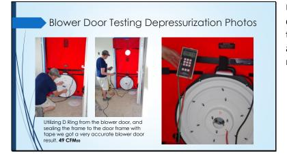
Utilizing D Ring from the blower door, and sealing the frame to the door frame with tape we got a very accurate blower door result. **49 CFM50**
