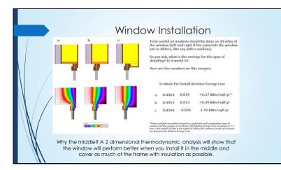
Window installation optimized. We put the window in the middle of the wall assembly, and insulated as much of the frame as possible to make sure the window would perform better than normal
