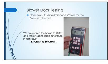
The use of Air Admittance Valves was used in many of the plumbing drains – to minimize plumbing penetrations. They work on opening when a sufficient pressure difference occurs allowing the water to fall and be followed by air. The pressurization test creates a similar situation, but the values didn't open enough to make a difference.
