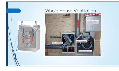
Air enters the ground loop heat exchanger where it is heated to 40 degrees. Then it goes into the air to air heat exchanger where it is heated to 66-68 degrees utilizing a cross counter flow heat exchanger. The outgoing air is thus cooled off keeping the heat inside the house.
