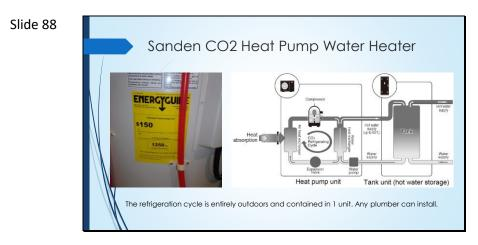
It is extremely efficient, and fairly simple to install. The heat pump heats water up to 160 degrees F and pumps it to the storage tank. At the outlet of the storage tank is a mixing valve. With 83 Gal of 160F water and a decent recovery efficiency we can supply a single shower with 1.5 hours of hot water (more when you use low flow heads and drain water heat recovery).
