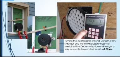
You can see the outside frame has not been fastened with the screw blocks. Oddly enough getting the assembly to be installed airtight was the hardest part – and it made a measureable difference. Once we did that we got the test down to 47 CFM50
