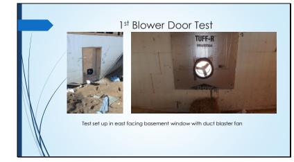
Used the duct blaster fan in a basement window for test
