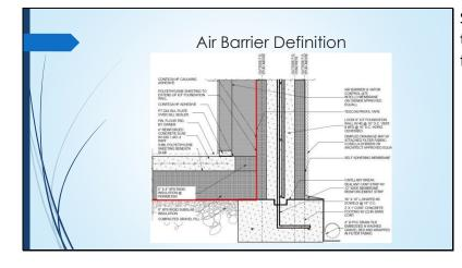
Sub slab radon barrier is sealed to the inside face of the ICF foundation
