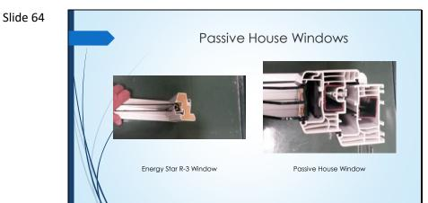
There is a noticeable difference in the construction of the windows! The window on the left is an Energy Star Rated Window, the window on the right is a Passive House Window
