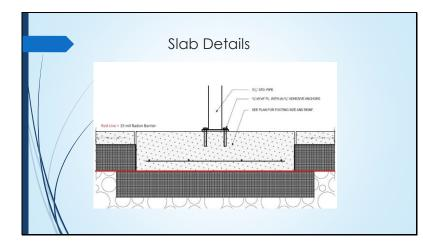
Sub slab air barrier. Keeping it simple!
