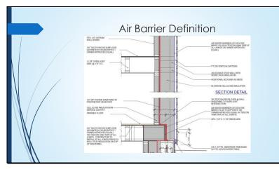
Interior wall is load bearing. The sheathing on the interior wall is our air barrier. This was chosen because is it protected from holes – either from the siding installation or from drywall installation. Keeping the air barrier intact is critical.
